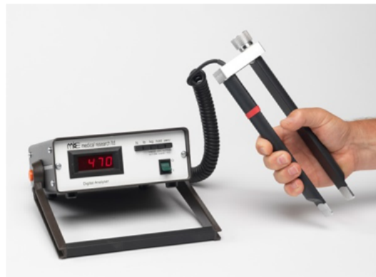
Figura 2.18: Digital Pinch/Grip Analyser MIE [77].
