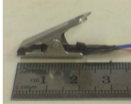
Figura 2.21: Pinch grip sensor [80].
